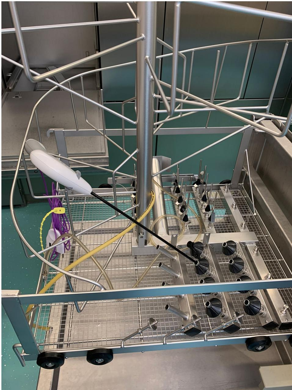
**Fig. 2** A LigaSure as placed in the rack in the instrument washing machine. The rack is used in human medicine for placement of anesthetic parts, hoses and connectors and slight adjustments have been made for the use of the vessel sealers. Water jets run through the cannulas where the tip of the vessel sealer is placed
